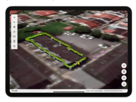
An area scan of 7m by 3.5m with a spacing of 0.25m was performed and the pipe was located. The team were able to see the pipe, its direction and depth and visualize it in Augmented Reality, enabling them to understand its exact location.
