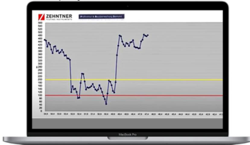
The retroreflection (RL) values are plotted against distance. The actual data is shown in blue colour. The values that are required by our national standard are also shown. These are 200mcd/m<sup>2</sup>/lx for new road markings (red colour) and 100mcd/m<sup>2</sup>/lx which is the minimum required value (yellow colour).
