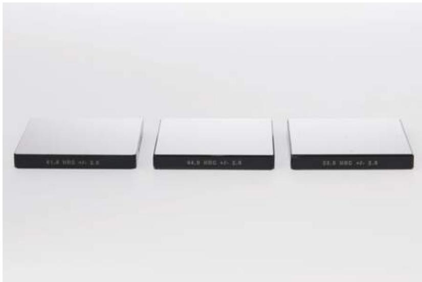
Equotip Portable Rockwell Test blocks
