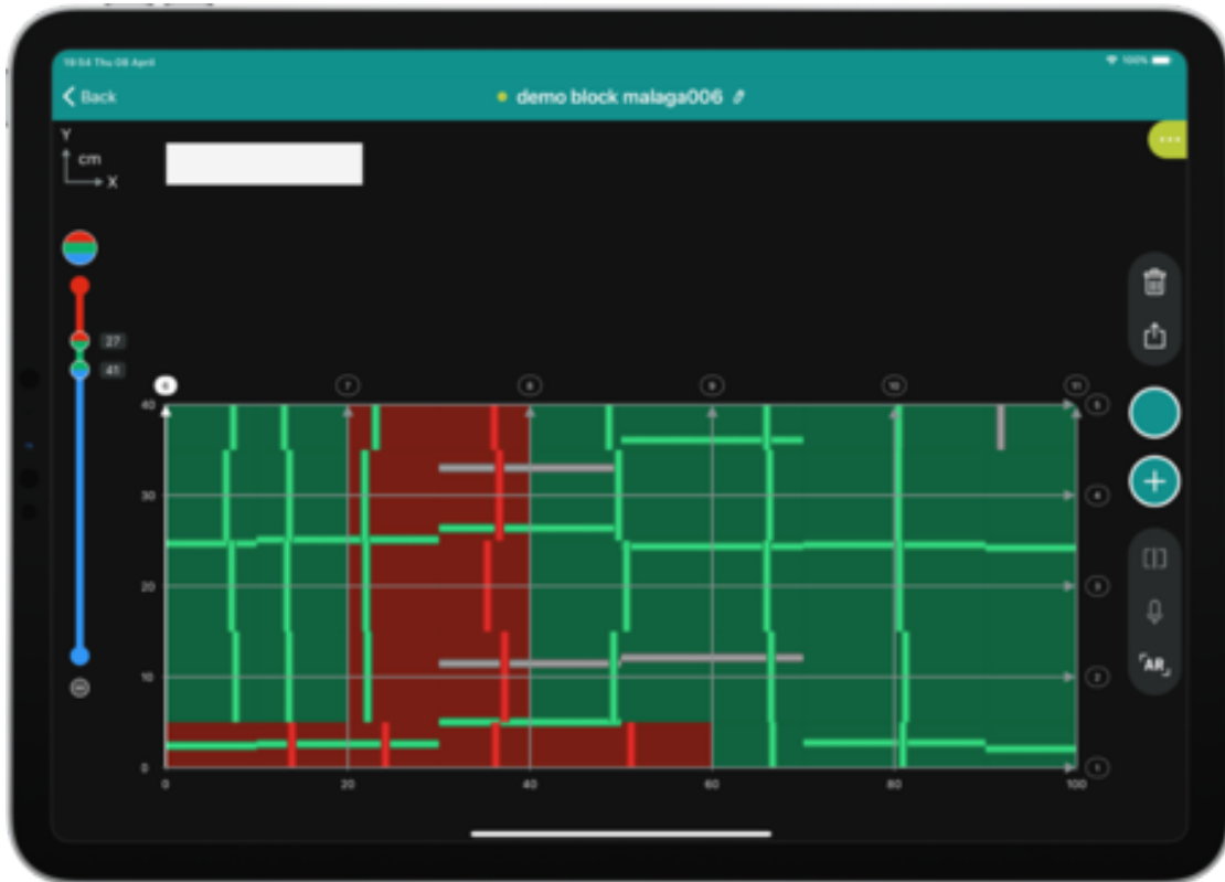
Concrete cover data using Profometer PM8000 Pro
