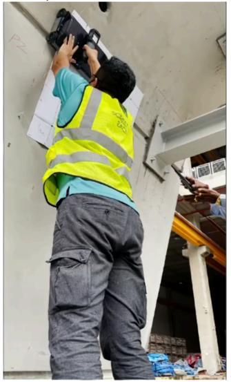
With the use of powerful data collection software, the <u>GP8100</u>, visualizes 3D data in real-time and the results can be presented in different views, like time-slice or as Augmented Reality (AR) view on the scanned area. Embedding the 2D or 3D results on the site using AR, allows us to capture the subsurface reality as is and create an intuitive report.
