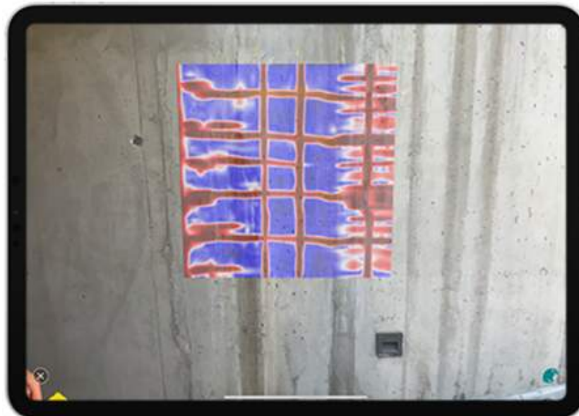
Area scan data shown on the iPad (left) and on the concrete surface (right)
