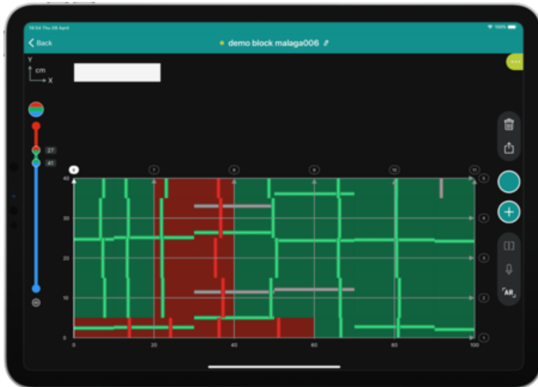
Concrete cover data using Profometer PM8000 Pro
