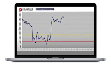
The retroreflection (RL) values are plotted against distance. The actual data is shown in blue colour. The values that are required by our national standard are also shown. These are 200mcd/m²/lx for new road markings (red colour) and 100mcd/m²/lx which is the minimum required value (yellow colour).
