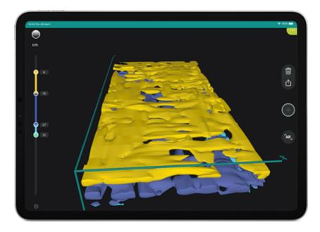
3D view of the top shift (yellow line) and mortal joint between second stone shift (dark blue line)
