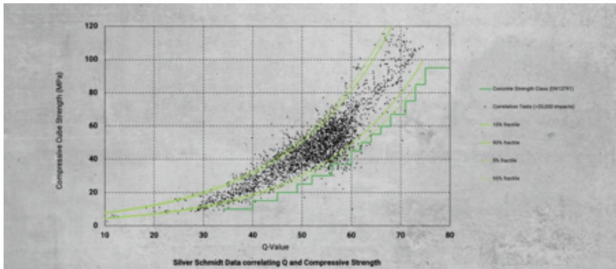
As with obtaining the result from crush tests, the rebound method is also statistical. When used correctly, it gives you more reliable, holistic, and much more cost-effective concrete strength estimation when combined with a few crush tests.
