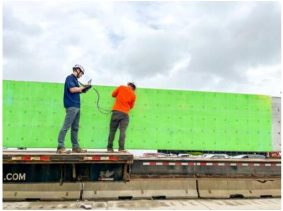
As a control test area, Durability Engineers' performed UPV on 12 ft by 2 ft direct transmission grid through the width of the beam (1.5 ft). The velocity readings ranged from 14,865 ft/s to 16,145 ft/s with an average 15,730 ft/s. This direct UPV testing was done to determine the baseline velocity of the concrete and to calibrate the measurements for indirect UPV testing.
