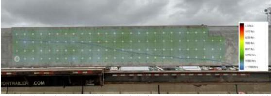
It was clear from the results that the velocities were similar throughout the measurement grid and do not indicate discrepancies or areas of weakness. Therefore, the UPV measurements indicated the beam has been placed monolithically and did not suggest the presence of a cold joint or discontinuity.
