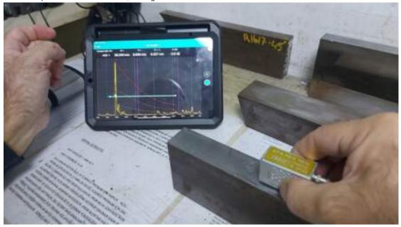
After the calibration the 2nd level has performed the inspection sharing video, in real-time.
