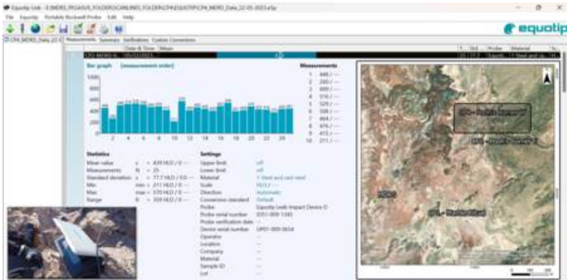
Fig.1: Example of some of the outputs acquired by the Equotip rock hardness in one of the stations (25 measurements in each station) of the scanline #4, located in Pooh's Corner (West side), Hanksville (Utah desert, USA).
